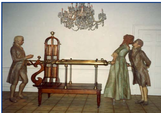
Fig. 2. Electrostatic generator for parlor amusements, ca. 1750. This apparatus is on display at the Smithsonian Institution's American History Museum, Washington, DC.
