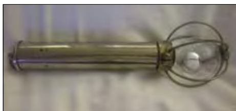
Figure 4. Mercury lamp used by Ralph Alpher while testing torpedoes in Puget Sound during World War II. If it was necessary for the testing crew to abandon their wooden boat, this lamp would emit a faint blue signal at night that could be seen by rescue teams.
